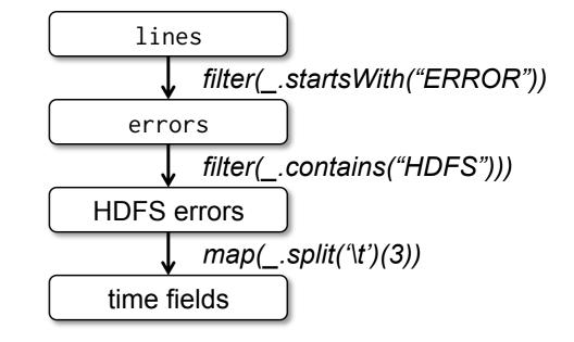
the lineage graph enables RDD re-evaluation in case of failure
